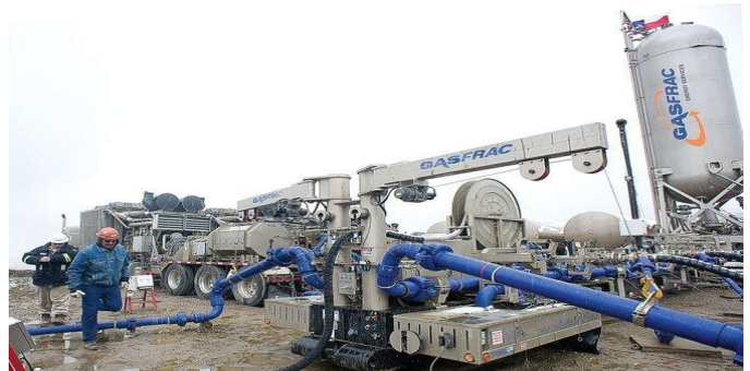
Picture 4.2.1: GasFrac Energy Services, Inc. Water-free hydraulic fracturing.
